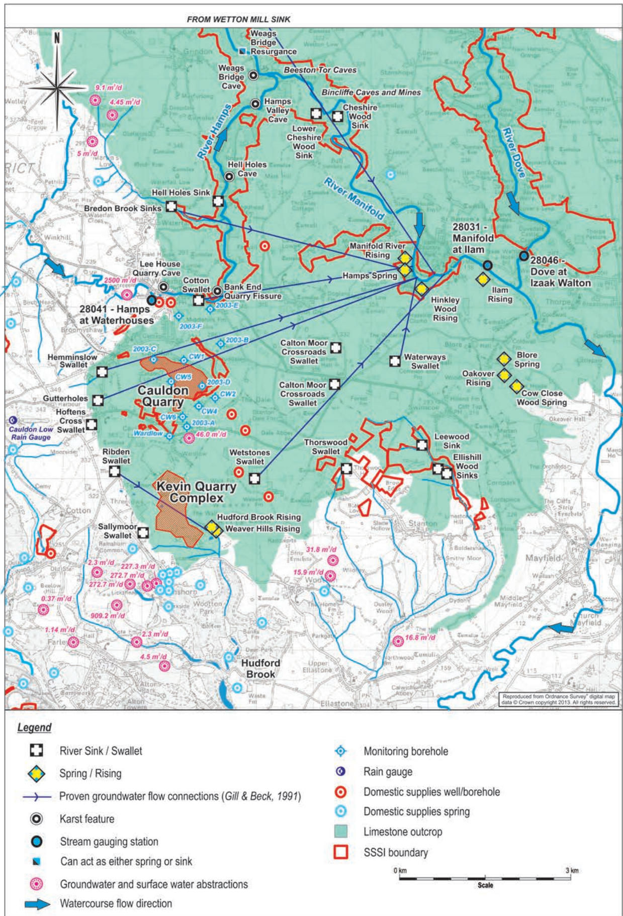
Figure 6. Hydrological and hydrogeological setting of Cauldon Quarry. The limestone outcrop area is presented, together with surface watercourses and known karstic features including river sinks, springs and established flow connections. Much of the rivers shown over the limestone outcrop are ephemeral in nature. The bulk of spring risings in the area are located just upstream of the stream gauging station on the River Manifold at Ilam.
