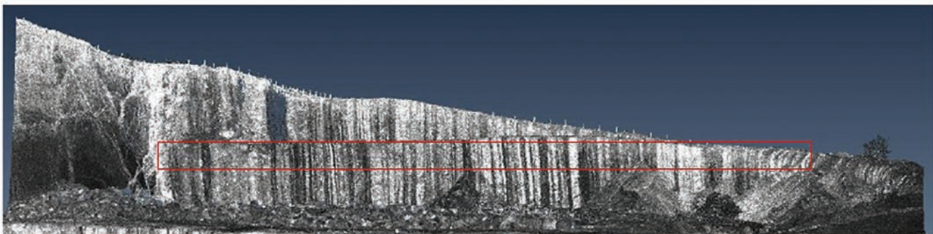
Figure 5. Colour scan; meshed and measurements made (manually) of a section of the face shown in Figure 4 from a range of 800m.
