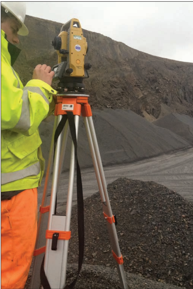
Figure 1. Total Station in use.
