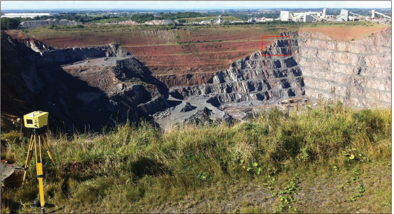
Figure 4. LiDAR scanner in use. The red rectangle indicates the scan shown in Figure 5.
