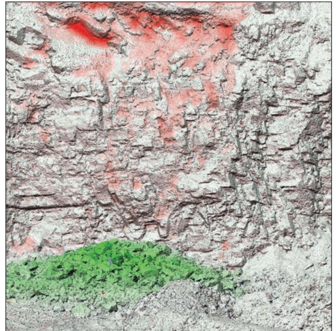
Figure 11. Comparison of pre and post rock-fall event LiDAR surveys. Red denotes areas of 'cut' and green denotes areas of 'fill'.
