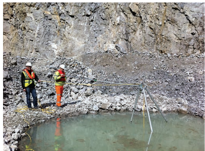
Figure 9. Tripod set-up over the cave opening, with the sonar instrument being lowered via the yellow cable.
