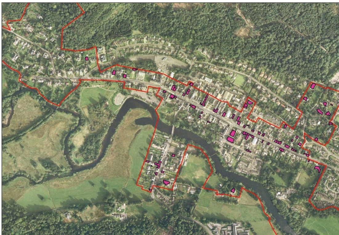
Figure 6. GIS view of an aerial photograph of Callander Conservation Area displaying the result of a cross query to identify all surveyed built sites with CONGLOMERATE (building stone) walling and CEMENT POINTING AND PATCHING (maintenance issue).
