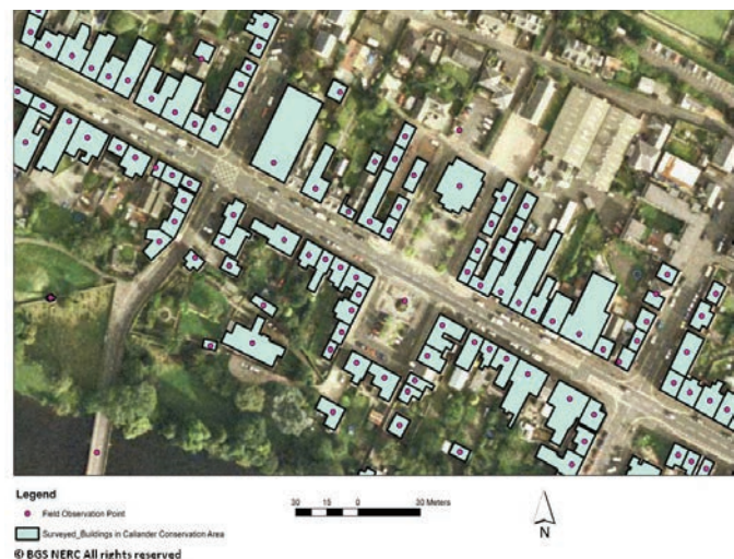
Figure 3. GIS view of an aerial photograph with georeferenced polygons representing the limits of each built site. Each polygon has a Field Observation Point, or unique reference number, used for identification and data attribution.
