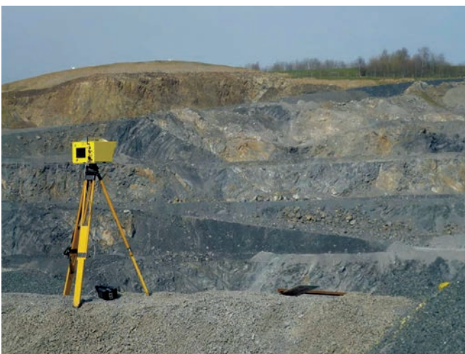
Figure 6. Photograph showing the laser scanner scanning the northern faces of Dolyhir Quarry.
