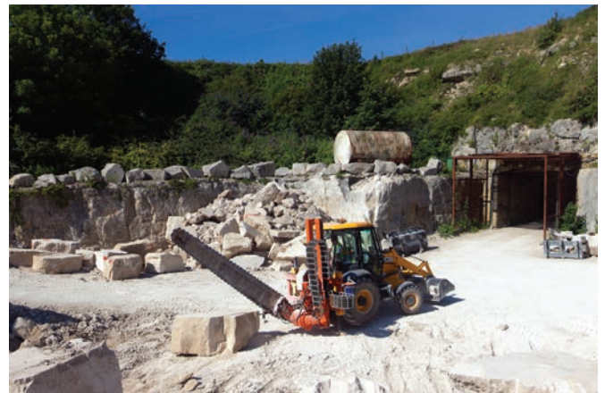
Figure 16. A JCB machine fitted with a Fantini chainsaw blade is used to “square” blocks taken from the mine faces, before they are sold.
