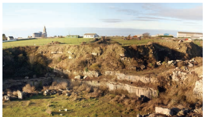
Figure 5. A remnant face at Jordans Quarry, pictured in January 2006, was selected for mining because it offered the most appropriate alignment for the cutting of tunnel portals and initial roadways with regard to the strikes of conjugate joint sets within the Freestone Beds.
