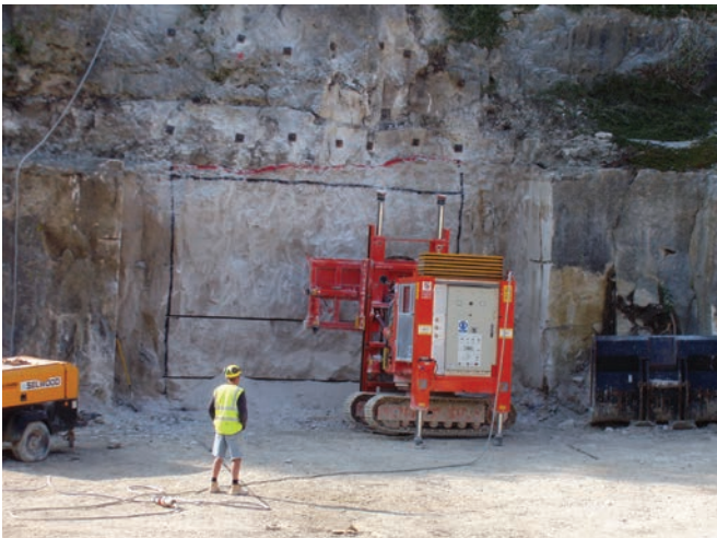
Figure 8. A Fantini GU50 mining machine being used to carefully cut the mine's first advance.
