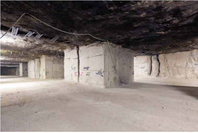
Figure 13. Very persistent master joints are routinely mapped and projected onto mine working plans, with the aim of providing an early warning of potentially difficult ground conditions in adjacent working areas.
