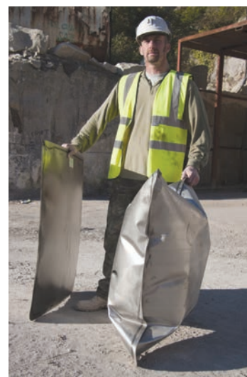
Figure 10. Un-inflated (left) and inflated (right) Hydro-bags. Hydro-bags are 3mm thick, 1m 2 high tensile steel envelopes that were originally developed for use in the Italian marble industry, these have now become a key part of Albion Stone's mining (and quarrying) processes on Portland, effectively replacing explosives. In use, each hydro-bag is inflated with water to a pressure of around 20 bar, producing a force equivalent to just over 200 tonnes.
