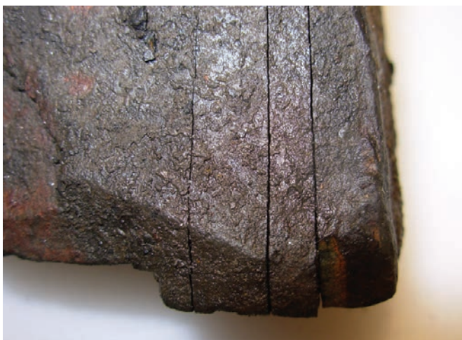
Figure 3. Aggregate particle from five-year old hardcore with laminations propped open with gypsum.
