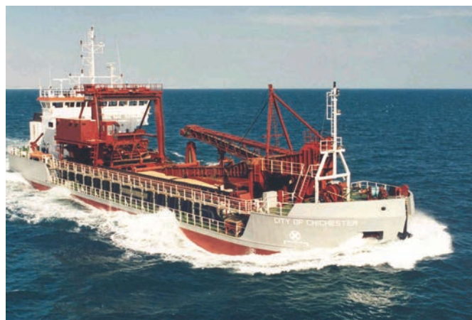
Figure 10. Tarmac Marine Dredging Ltd's dredger "City of Chichester" returning to Southampton wharf having dredged a cargo of sand and gravel. Built in 1997, the purpose built vessel has a cargo capacity of over 2200 tonnes and can dredge in water depths of up to 35 m.
