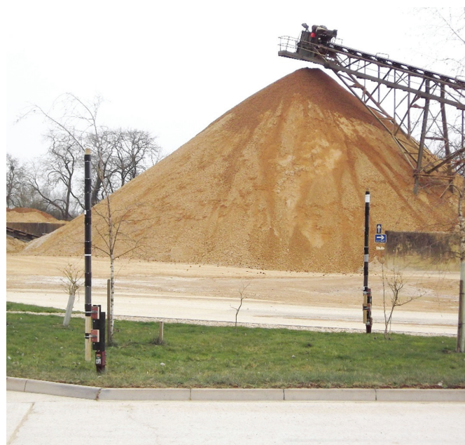
Figure 6. Two multi-height dust monitors adjacent to a quarry haul road.
