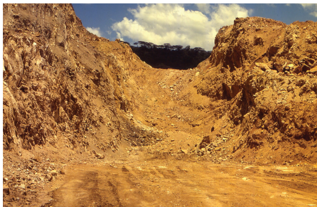
Figure 7. Photograph showing one of the open pits at the Kimwarer fluor spar mine in Kenya. Ore is extracted from seven separate open pits and is blended. Surficial oxidation has produced fine-grained goethite that colors the ore yellow.
