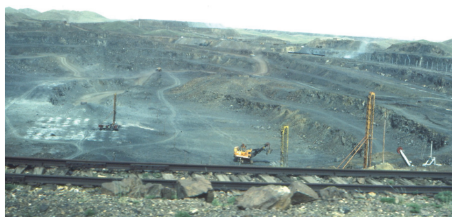
Figure 12. Photograph showing the east open pit at the Bayan Obo magnetite-hematite-REE mine, Inner Mongolia, China, which has been mined to a greater depth than the main open pit. Mine equipment for scale.
