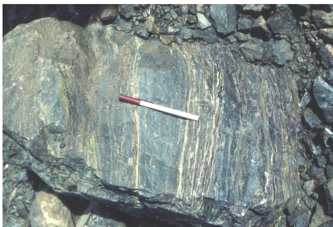
Figure 14. Mine photograph of a hand specimen of bastnaesite-rich iron-REE ore. This specimen is typical of REE-rich ores called striped ore by mine geologists. Bayan Obo magnetite-bematite-REE mine, Inner Mongolia, China. Red and white pen for scale.
