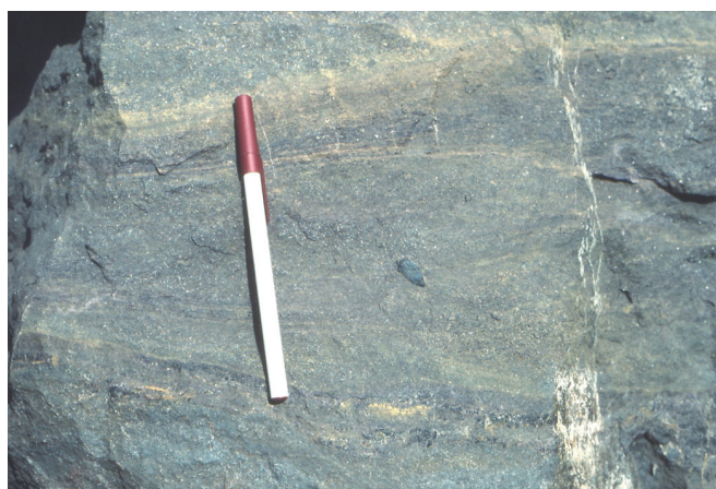
Figure 13. Mine photograph of a hand specimen of monazite-rich, iron-REE ore. The presence of abundant monazite gives a brownish cast to the ore. Bayan Obo magnetite-hematite-REE mine, Inner Mongolia, China. Red and white pen for scale.
