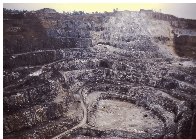
Figure 8. Photograph showing the open pit at the Cajati apatite mine, Brazil. The darker areas of rock are earlier intruded jacupirangite and the lighter areas are subsequently intruded carbonatite. Mine equipment for scale.
