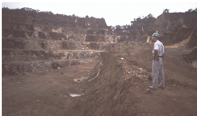
Figure 6. Photograph showing the open pit at the Mato Preto fluor spar mine, Brazil. The lighter areas are carbonatite and the darker areas are tinguaitite dikes. The fluor spar mineralisation has been interpreted to have replaced tinguaitite and cannot be distinguished at this scale. Mine benches are about 13m high.
