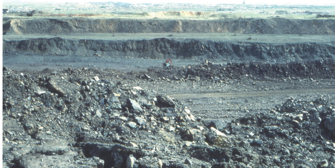
Figure 11. Photograph showing the main open pit at the Bayan Obo magnetite-hematite-REE mine, Inner Mongolia, China. The ores are mined primarily for the iron minerals; magnetite and hematite. The REE minerals are recovered as by-products. Mine equipment for scale.
