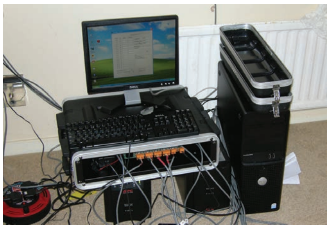
Figure 10. Bespoke blast monitor situated at Incline Side property.
