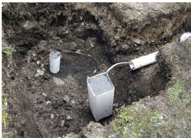
Figure 9. Tri-axial array and trigger geophone located outside the property prior to burial.
