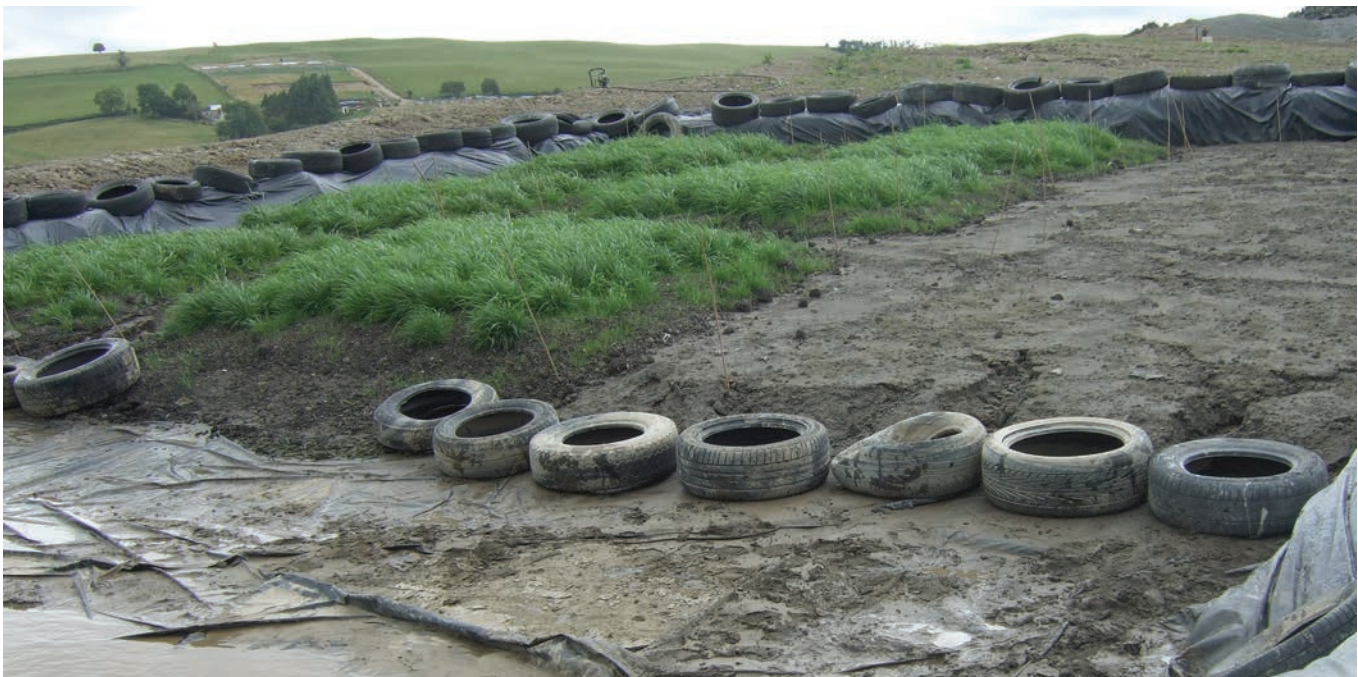
Figure 3. The benefits of adding PAS100 at Bryn Posteg; on the left hand side PAS100 has been added but not on the right hand side where seeding has failed in the lead-rich mineral waste.
