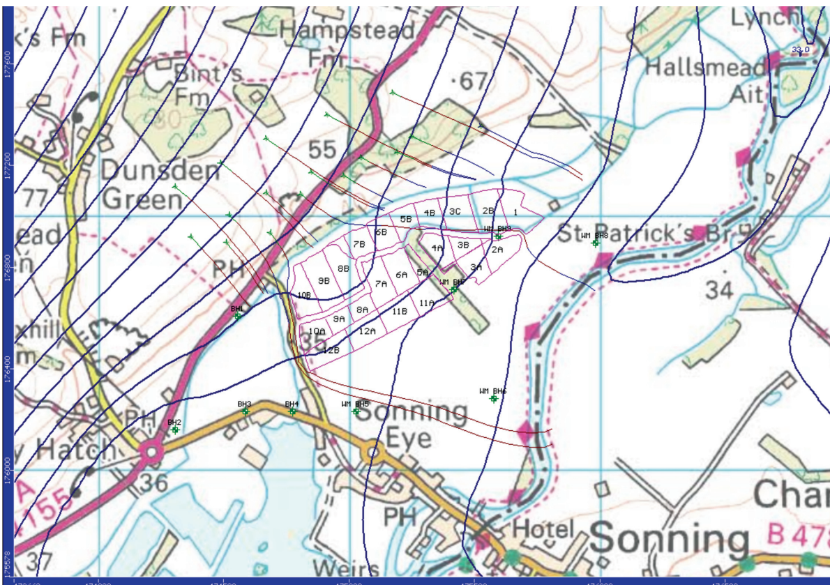
Figure 7. Post-development scenario groundwater flow paths in the chalk shown in relation to the extraction phases. (blue lines = groundwater level contours; red lines with arrows = particle flow pathlines; pink cell boundary lines = extraction phases within Area C).
