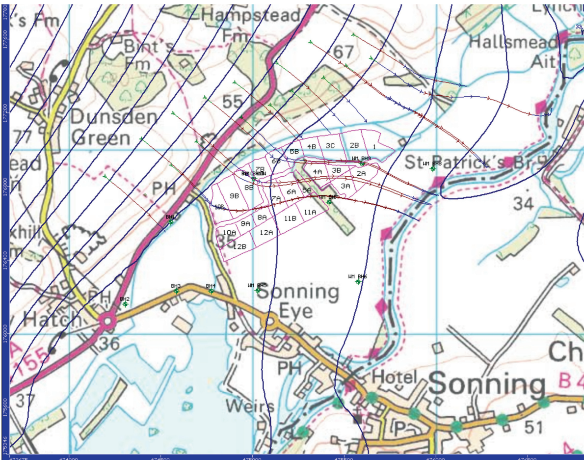
Figure 6. Pre-development scenario groundwater flow paths in the chalk shown in relation to the extraction phases. (blue lines = groundwater level contours; red lines with arrows = particle flow pathlines; pink cell boundary lines = extraction phases within Area C).
