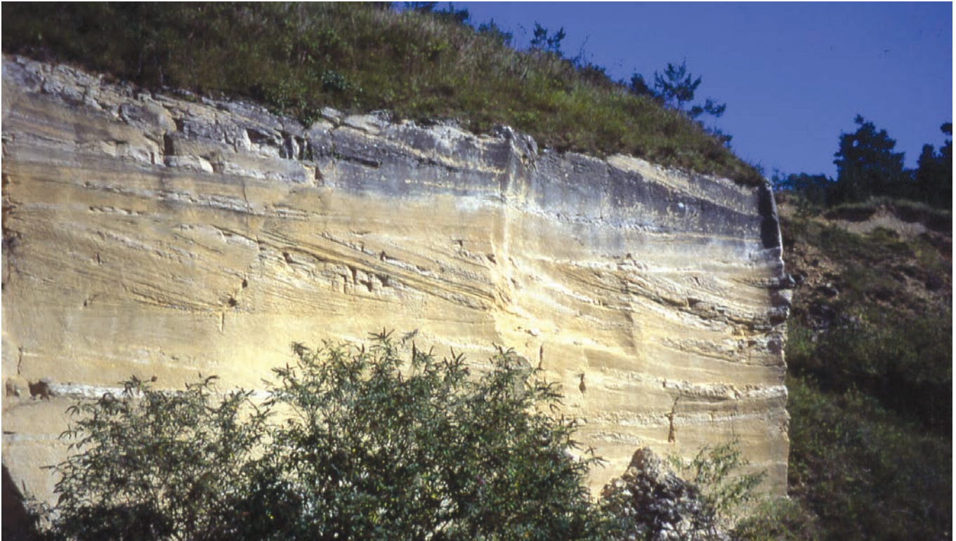
Figure 11. Creully, the most prolific of the 'soft rock' quarries operated by the Quarry Group RE in Normandy: photographed in 2001, showing face some 4 m high cut through Mid-Jurassic cross-bedded bioclastic limestones. From Rose & Pareyn (2003), courtesy of the Geologists' Association.
