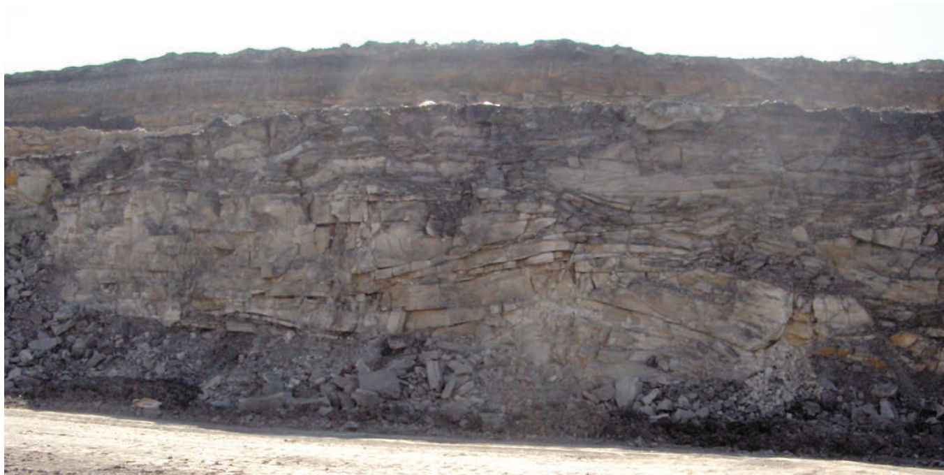
Figure 4. Penecontemporaneous slumping in inter-seam strata including contorted bedding and intra-formational shear surfaces inclined in different directions. The face height is approximately 12m and the open cast coal site is in Scotland.
