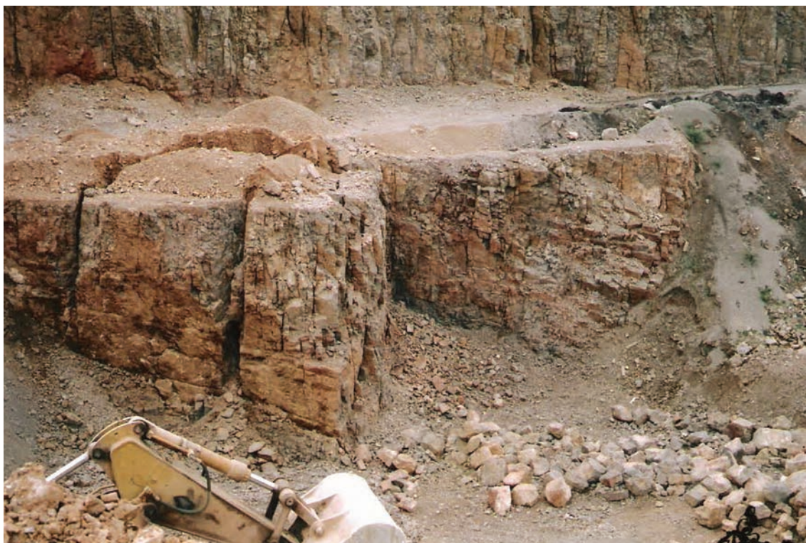
Figure 5. Sliding movements occurring on a clay way-board in a Carboniferous Limestone quarry in South Wales. The inclination of the strata and the location of the way-board are visible above the backhoe boom; the vertical and lateral displacements were approximately 1m and 2m respectively at this stage of movement.
