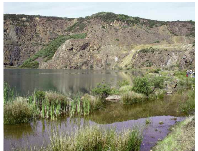
Figure 5. Part of the quarry with the centre of the photograph showing a promontory that includes a large composite NW-SE quartz vein with attendant kaolinisation. The quarry sump has subsequently been lowered by 9m.
